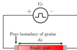
Pore pressure increase due to Plasma Formation is sufficient to induce fracturing in granite.
