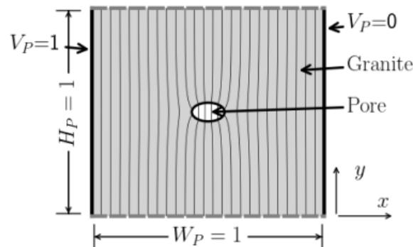
We use this model to calculate the electric field distribution: (1) across the sample to distinguish which regions have the highest electric field values and (2) across one single pore of different fluids, shapes, sizes, and orientations.
