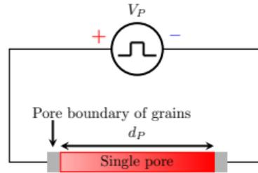
Pore pressure increase due to Plasma Formation is sufficient to induce fracturing in granite.
