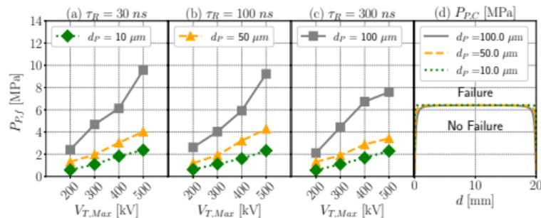
Single pulse is enough to cause damage in rock of 100  $\mu\text{m}$  pore size (e.g., tuff or sandstone). However, A few pulses are necessary to cause damage in rock of pore sizes smaller than 100  $\mu\text{m}$  pore size (e.g., granite). Shown experimentally by [Lisitsyn et al. (1998)].
