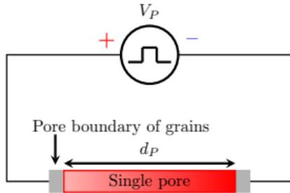
We use **ZAPDOS application** to simulate the plasma formation in a single pore and calculate the deposited electric power in the pore.
