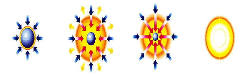
1) Atmosphere formation: Laser beams rapidly heat the compressed by the rocket-like surface of the fusion target forming a surrounding plasma envelope.
