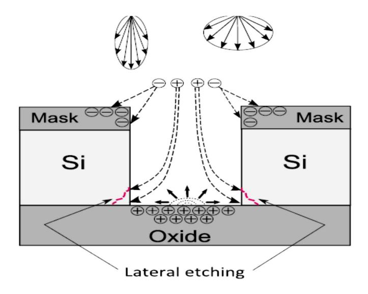
The defect generation due to charge build-up and UV photons were found to occur at a time constant of  $10^{-3}$  s during plasma etchings.
