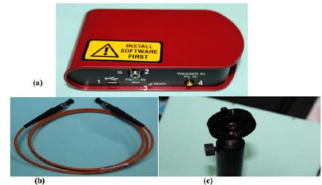
Figure (2.11) A) the used spectrometer: 1. USB port 2. Fiber input 3. Status LED 4. Trigger Input B) Lens C) Optical fiber.
