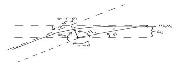
Collision between an electron and a heavy ion (for more details see lonospheres Physics, Plasma Physics, and Chemistry P75)
